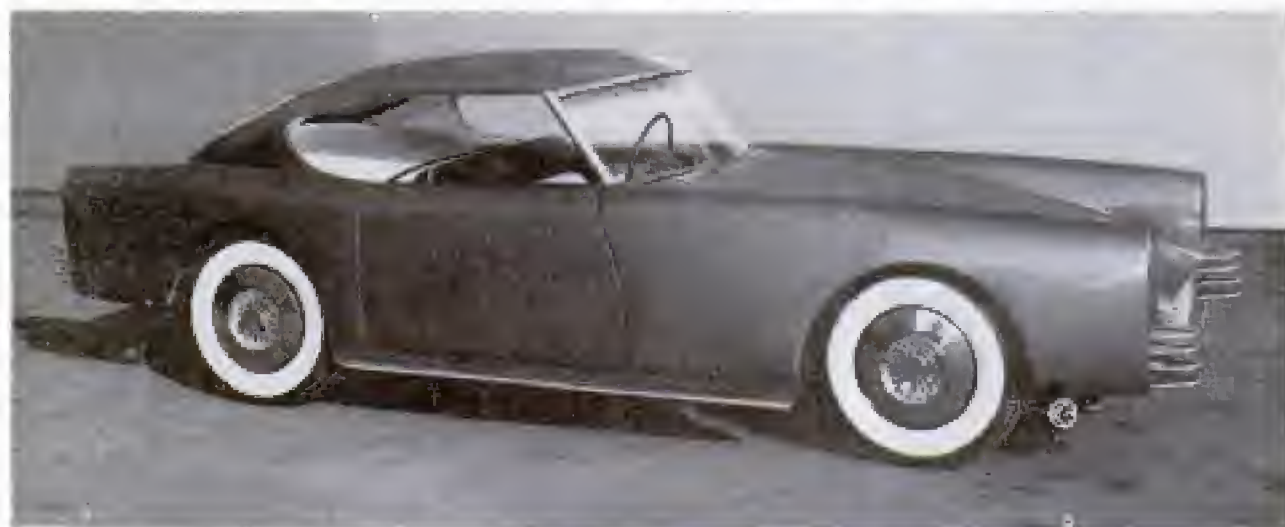
Everett coupe has tubular steel frame, uses the tubing to carry water from engine to rear-mounted radiator
